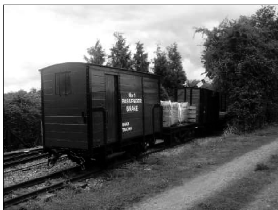
Figure 5. A former Trecwn brake van now re-gauged for use on the North Gloucestershire Light Railway at Toddington, May 2019.
