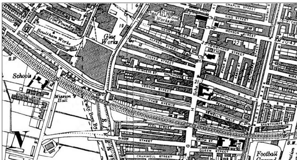
Fig 3. An enlarged extract from 1930 6 inch OS map, showing where Great Gowts Tunnel passes under the upper river Witham and the road, between Coulson Road to the west, and Boultham Avenue to the east. It was part of a scheme to separate upland from lowland waters, and carried lowland drainage into the Sincil Dike, which was extended to discharge via the South Delph into the Witham below Bardney Lock.
