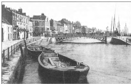
A card postmarked 1905 showing two 'clinker-built' Parrett Barges moored above Bridgwater Town Bridge shortly before high tide. In the previous century similar craft would have traded to Langport. Note the 'drag-chains' on the foredeck, which could be paid-out over the bows to slow or stop the vessel on the tideway. The absence of a fore-hatch suggests that the crew's accommodation beneath the foredeck could not be accessed when the vessel was fully laden. (RCHS Collection)
