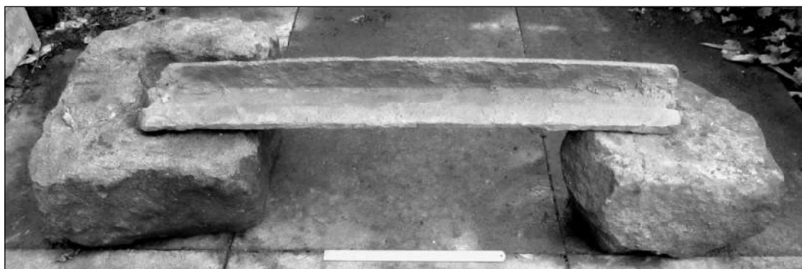
Figure 5. A plate rail cast at Butterley to Outram's pattern and used on the company's own line at Codnor Nether Park, Derbyshire. The stone sleepers are from John Rennie's Lane End line, Staffordshire. This plateway was built to Outram's design using Butterley rails. The height of the flange is greatest in the centre of the rail for increased strength. (Author, scale: 12 in rule)
