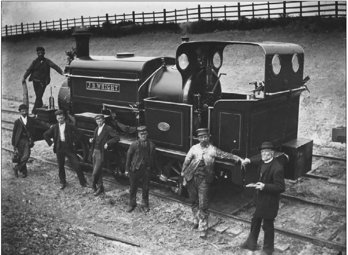
Figure 3. In the cutting at Cowley, near Twyford, Bucks, S W A Newton photographed this gleaming Manning, Wardle saddle tank J.R.Wright (MW1228 of 1895) which belonged to the contracting company Walter Scott & Co.
